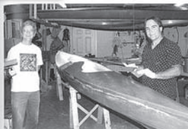
Applying a protective coat of epoxy
